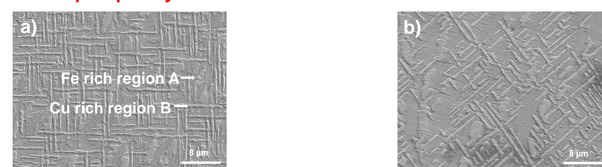
Fig: SEM image of AlCuFeMn HEA oxidized at a) 500°C b) 1000°C for 50 hours respectively.
