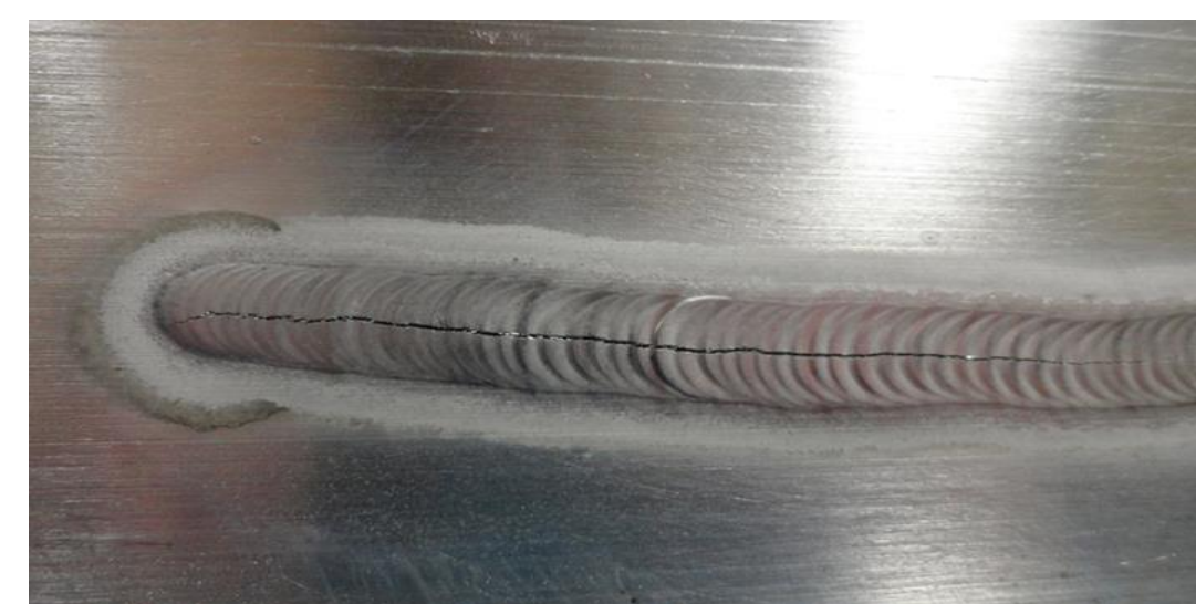
Fig: Weld crack in AA6061 base plate during TIG welding (Courtesy: Welding Productivity).
